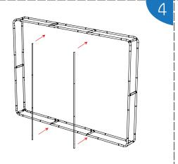
Install the middle tube to finish the frame
