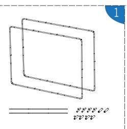
Put both horizontal tube connect with same label in to a frame, as the picture shown, and prepared the middle tube
