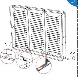
Hang the LED light into the frame sequentially, beware the direction of the LED panel
