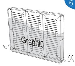
Set up graphic to the frame. (Light power line should be out from holes in graphic; If it's single side printing, the LED direction should face the back of the graphic to achieve better effect)
