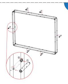
Install the rest horizontal connectors
