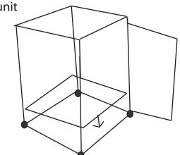
Note: The wooden floor panel is the panel with all the hardware attached on the underside. Remove all hardware from the panel before assembly
