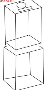
**Step 11**: With all doors open on both the top & bottom cases, proceed to connect the wiring from the bottom case to the wiring on the top case.
