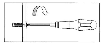
4-B) Press down firmly on the head of the screw with a screwdriver and turn the screw clockwise until the barrel crimps against the inside of the wall.
