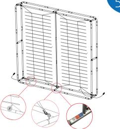
Hang the LED light into the frame sequentially, beware the direction of the LED panel
