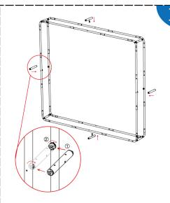
Install the rest horizontal connectors
