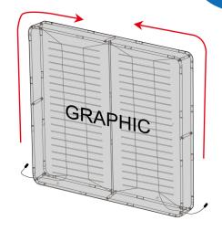
Zip the zipper. Fix the whole frame into the base and lock the slider with allen key
