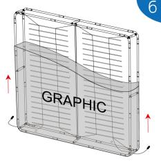
Set up graphic to the frame. (Light power line should be out from holes in graphic; If it's single side printing, the LED direction should face the back of the graphic to achieve better effect)
