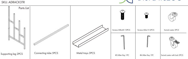
STEP 1. Assembly the castors on the two supporting legs, the casotrs with lock are in the back of unit, as shown above.
