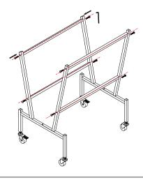
STEP 3. Assembly the metal trays to the frame by using M6\*15 screws and tighten them with #4 Allen key.
