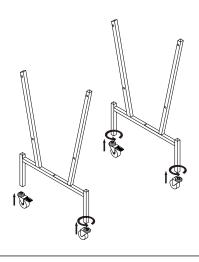
STEP 2. Assembly the supporting legs with connecting tube by using M8\*40 Screws and tighten them with #5 Allen key.
