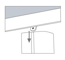
1. Slide the two (2) connector plates down the groove of the pole to the desired height
