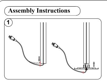
1.Remove the wire clip on the end, slide the Charging Set Steel Base from the end.
