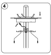
4.Slide the Acrylic Charging Set from the top, connect the power cord with the adapter inside the Acrylic Charging Set, and then fixed with the Charging Set Steel Base with M3x5 Machine screws.
