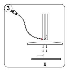
3.Connect the Pole, Base and weight piece as in the diagram.
