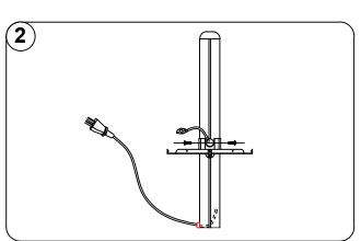
2.Fix the Charging Set Steel Base with the holes on the pole with M4x18 screws, tighten the screws on the connectors in the grooves.
