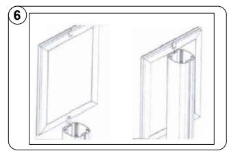
6. Slide the (4) Connecting plates on the back of (2) snap frames into the grooves of pole set and adjust to desired height.
