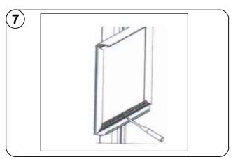
7. Open the upper covers of horizontal sides; Tighten the screws on the tops and bottoms of the frames.
