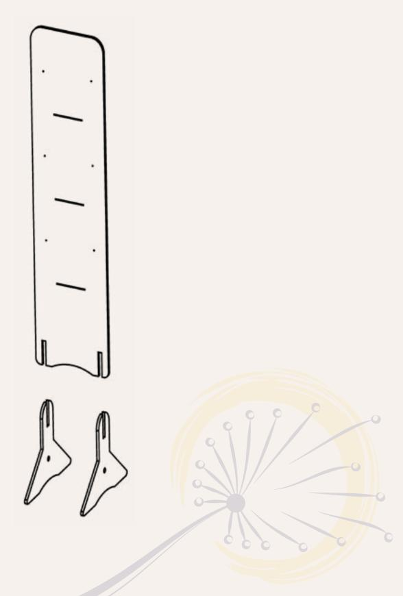
1. Slot feet into grooves at the base of the back panel.
