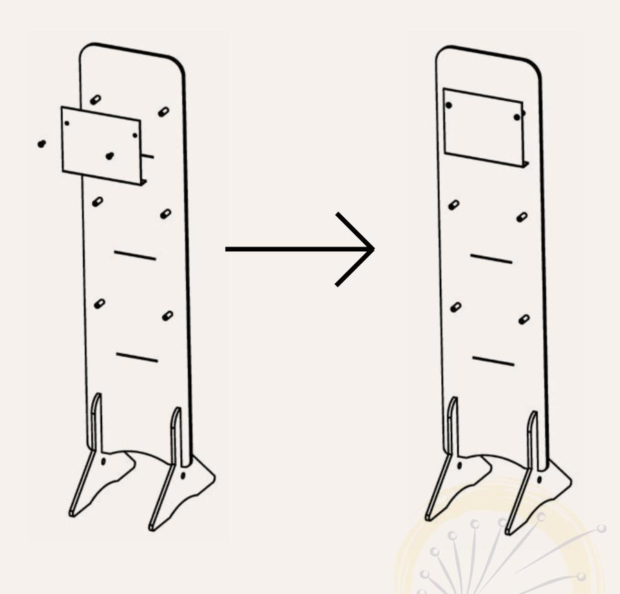
3. Affix pocket to back panel using pegs to secure. Slot peg into tube. (x2)
