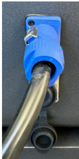
2. Align the notches of the power cord with the outlet, then insert.
