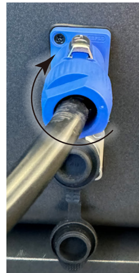
3. Press down the metal tab and turn clockwise.
