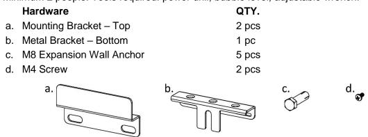
Step 1: Assemble the Metal Bracket (b) to the bottom back-side of the white board with (2) M4 screws (d), as shown below. Do not tighten the screws.
