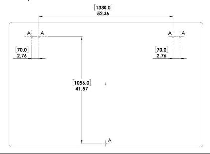
Step 3: Insert the (5) expansion wall anchors (c) into the holes drilled in step 2, then unscrew the M8 Hex screw from the anchor sleeves. Make sure all anchors are flush against the wall. See below:
