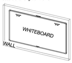
Step 7: Horizontally slide the assembled bottom bracket at the back of the whiteboard, until the wall anchor can be seen through the cutout on the bracket. Fix the bracket from the back by tightening the 2xM4 screws on the back of the whiteboard.
