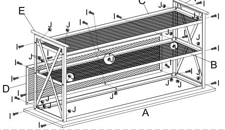
Step 3. Carefully bring the assembled cart to its upright position. Unpack and place Mesh Basket (G) onto the middle shelf as shown.
