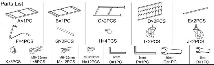
Step 1. Assemble Side Frames (C) with Wine Racks (D), Middle Shelf (B) and Metal Bars (E) by using Screws (L, M, N) and included Hex Key (O, P) as shown below.
