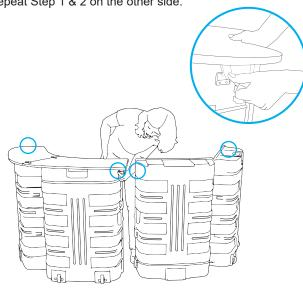
3. Move 2 assembled cases next to each other and join them by locking the latches underneath the countertops. Wrap the PVC kickplate around the bottom to cover wheels. Attach the hook and loop strips on the ends of the kickplate to the corresponding pieces inside the case.
