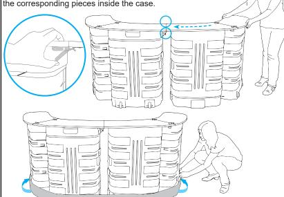
4. To attach the printed graphics, remove the protective paper on the adhesive backing of 4 hook and loop strips and apply to the back side of the graphics. Be sure the attached strips match The assembly is finished. with corresponding pieces inside the case.
