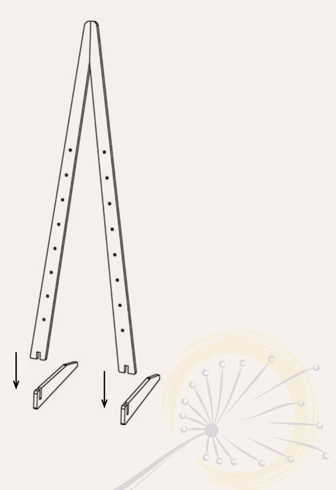
1. Insert standing pieces into the base pieces by aligning notches and fitting together.
