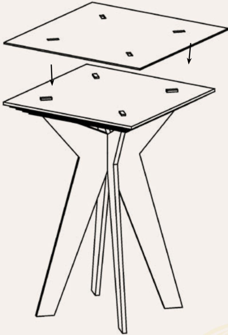
4. Press-fit the plywood table top onto the unit. Press firmly to secure the unit and ensure stability. Assembly is complete.
