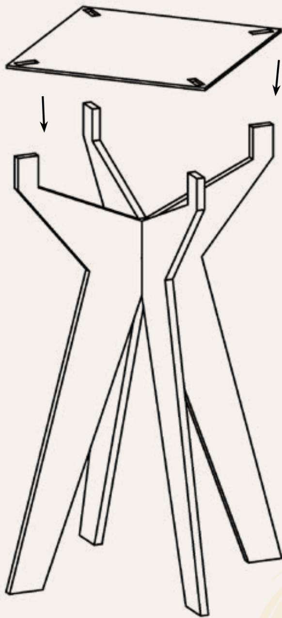
2. Press plywood table bottom piece onto legs by gently fitting the holes over the top portion of the legs.
