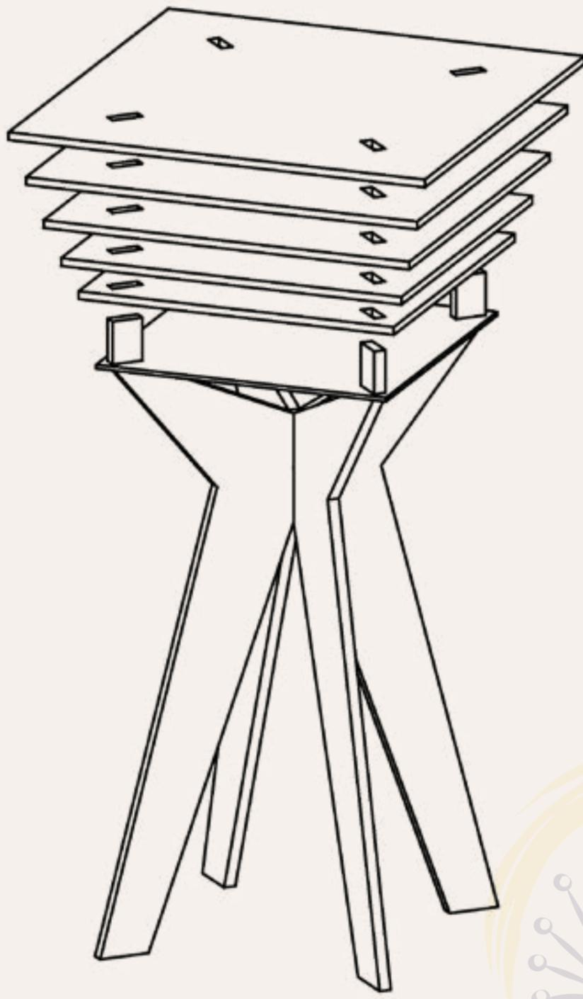
3. Press the five honeycomb cardboard pieces onto the table base. Be gentle with the cardboard pieces to prevent damage.
