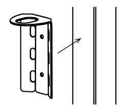
Wall Mounting Option: Use 2 holes in backside of bracket for wall mounting. Hardware not included.
