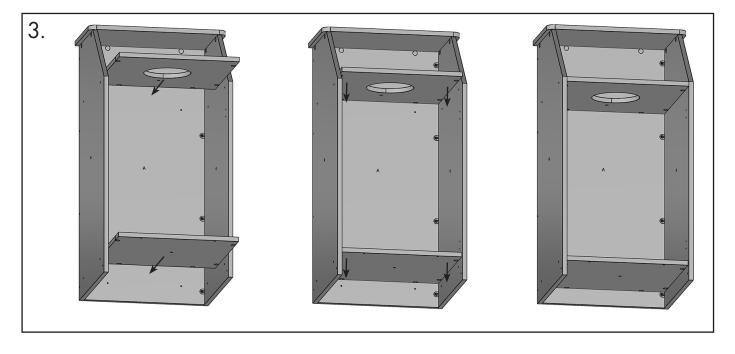
3. Insert the loading panel (E) in between 2 side panels and slide down as shown. Turn cam locks clockwise to fix. Do the same to the bottom panel (D).
