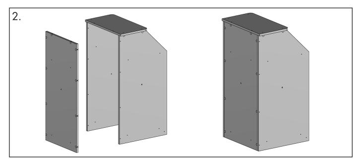
2. Connect the back panel (A) with the panel assembly finished in Step 1.
