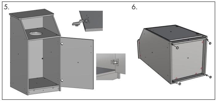
5. Attach hinges to Door (G) using pointed screws. Attach the door to the side panels.6. Insert glides (L) to the bottom of the side panels and middle panel and use a rubber mallet as needed.
