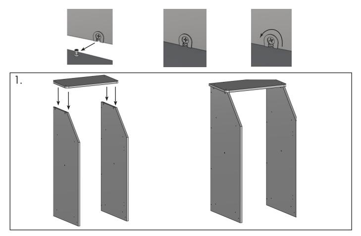
1. Connect the top panel (H) with 2 side panels (B&C) by locking the cam locks with cam screws.
