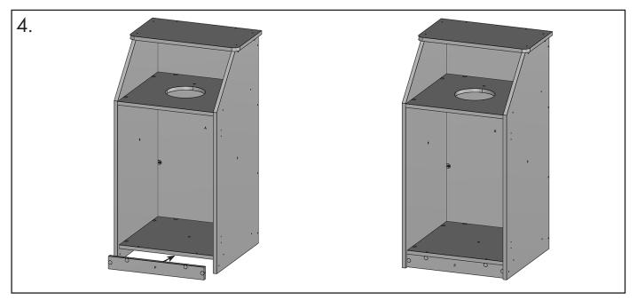
4. Attach the kicker panel (F) to the bottom as shown, and fix the panel by tightening the cam locks.
