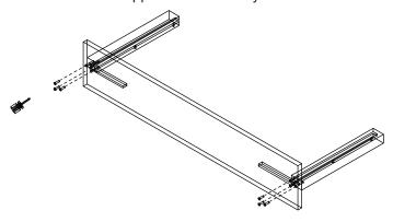
2. Move the assembled base to its standing position. Slide the Acrylic Panel (A) down with the bottom inserted into the cutouts in the base, and then fix it with 2 M4 Set Screws (D) and Allen Key (F) as shown.
