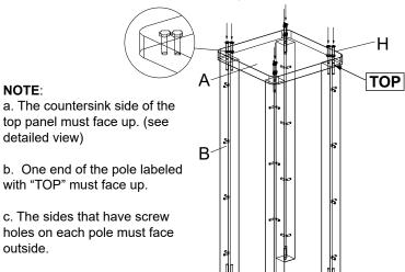
STEP 2. Hold the poles and the top panel, and carefully turn the assembled frame upside down.
