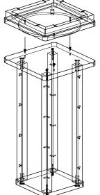
STEP 5. Carefully place the assembled unit on its standing position. Assemble Small Shelves (D) and Large Shelves (C) onto the display body with M4 screws - Short (I).
