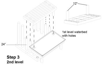
Position 2nd level panel over 24" legs and 12" legs over 1st level waterbed as shown. Slide 12" legs into holes of waterbed. Push down until 24" legs rest on top of socket.
