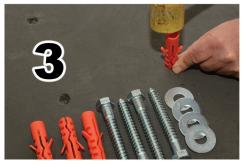
• Use a rubber mallet or hammer to stuff expansion plugs into the drilled holes
