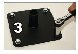
• Place the base plate over the four holes and use a socket wrench with a 3/4" drive to thread all four bolts
