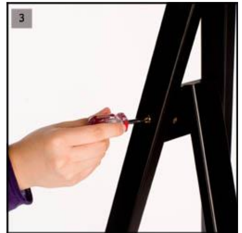
3 Tighten the screws from the side to hold the easel together
