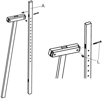
Tips: Adjust the lock nut with a flat head screw driver to help threading in the hex screw.
