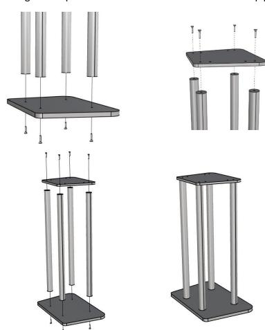
If you also purchased FLTCTTOP, assemble the entire lectern by placing the top onto the base and securing using 4 bolts provided.
