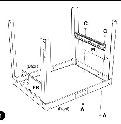
Take the top shelf of your metal cart and lay it flat. Collect parts: **FL**, **FR**, **A** & **C**. Push Screw **A** through the hole at the top of the shelf. Lay bracket **FL** & **FR** on top of screw **A**. Take nut **C** and fasten with a screwdriver and pliers, do not tighten fully until shelf is attached.
