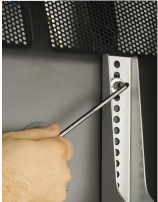
Line up long brackets with appropriate holes on back of television and screw in with provided screws.
