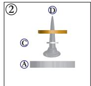
Flip the brass washer over and assemble the unit as pictured.
