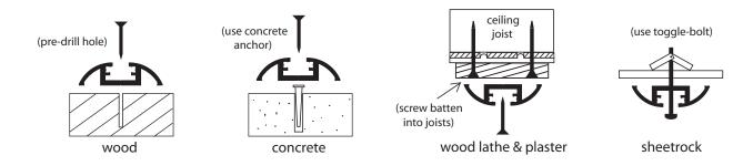
3. After deciding on the best way to mount the rails, screw them into your walls or floor and ceiling. To transfer measurements from ceiling to floor it is helpful to use a plumb bob.
