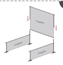
Assblem the upper and bottom vertical pipe of backwall together
