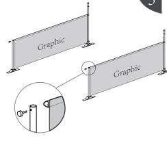
Connect vertical pipe to horizontal pipe of halfwall graphic, fix the screw
