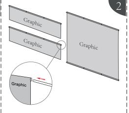
Put the each group horizontal pipe into the top and bottom of the graphic
