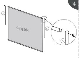
Connect upper vertical pipe of backwall to graphic, fix the screw
