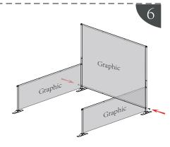
Fix screw of bottom horizontal pipe with bottom vertical pipe of backwall
