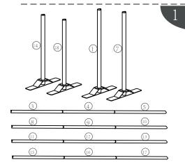
Put the vertical pipe into base, and fix the screws on the bottom; Contect the 4 group horizontal pipe as the instruction
