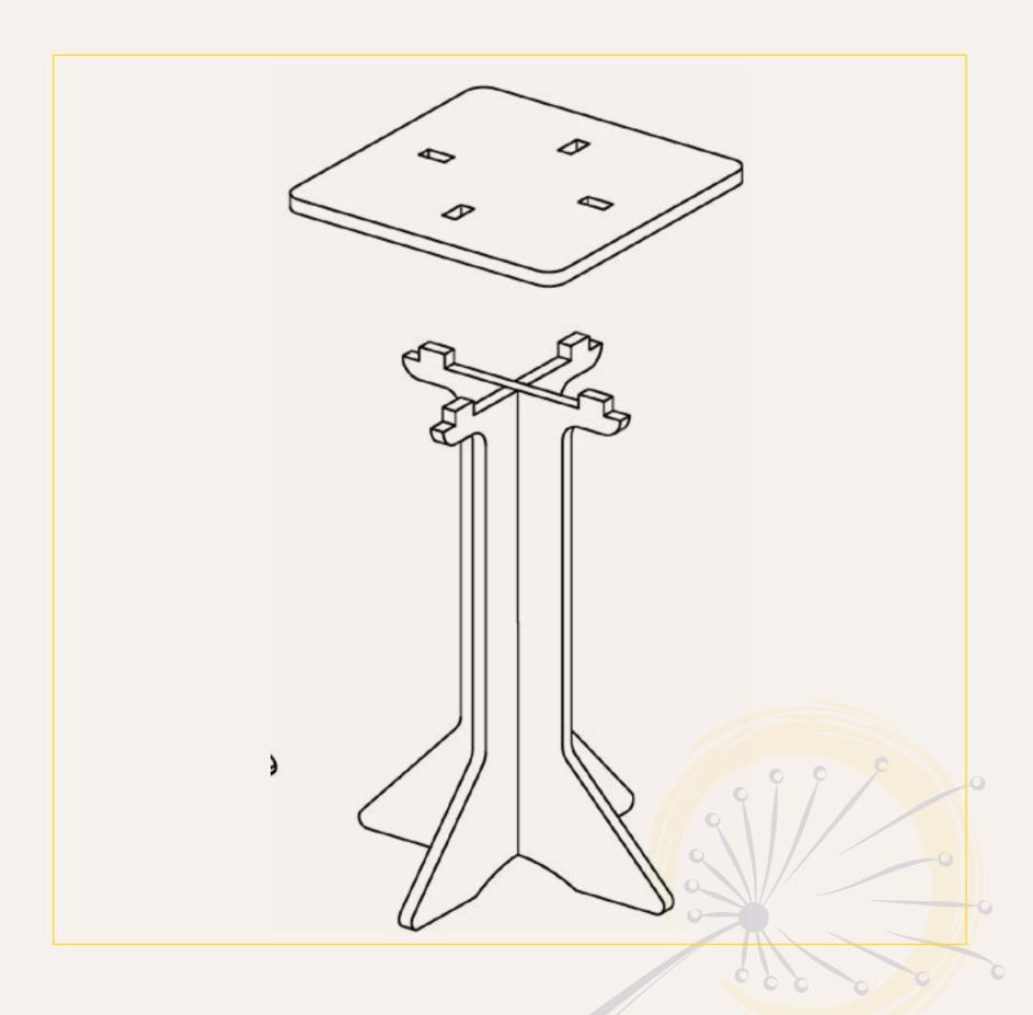
2. Place the tabletop on the top of the base. Insert the tabs into cutouts on the tabletop.
