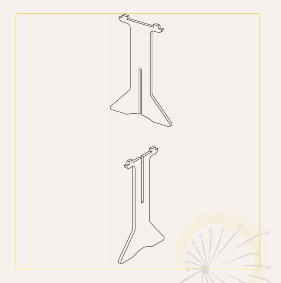
1. Assemble the pedestal base by inserting one base board into another at the cutout. Press down until the bottom feet are flush.
