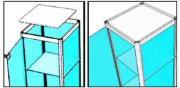
Slide 1 peg (H) into the slot in a corner post, then tighten them with a screw driver. Do this at all 4 corners.
