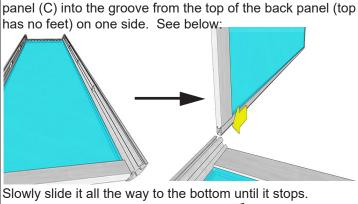
1. Place the back panel (A) on a soft work area. Slide 1 side
