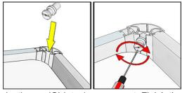
Insert 1 plastic cap (G) into 1 corner post. Finish the assembly by doing this for all 4 corners.
