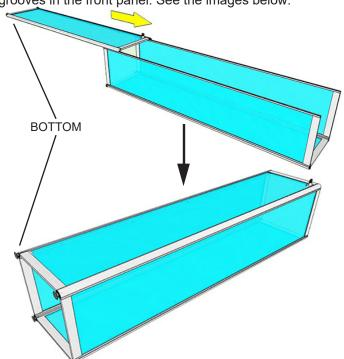
5. Place one wood board (F) at the bottom inside the display
