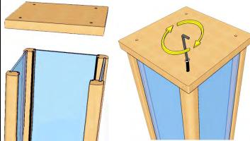
5. Push the plastic inserts into the top and bottom panel, and place the glass door holder (I) in place as shown below. Install the 2nd holder at the top the same way.
