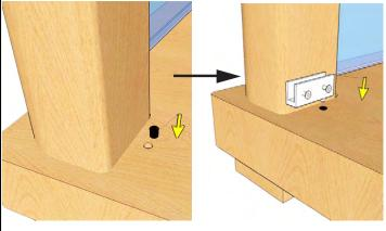
6. Carefully lift the glass door panel (D) and insert both ends into the metal brackets assembled in Step 5. Adjust the glass door to its best fit then tighten screws with screwdriver. *Tips: Open and close the glass panel to check if the door can move freely. Adjust as needed.*
