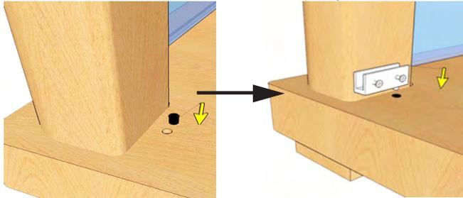
6. Carefully lift the glass door panel (D) and insert both ends into the metal brackets assembled in Step 5. Adjust the glass door to its best fit then tighten screws with screwdriver. Assemble glass doors on both sides.
