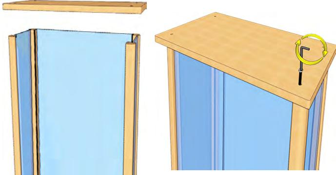
7. Assemble the door lock (I) by securing it on top of the glass door. Test the lock after assembling.
