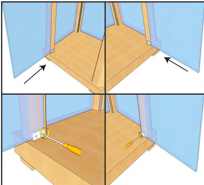
9. Insert the glass seal starting from 1 corner outside the display case. Apply silicon glass seal provided to all edges of the back and side glass panels.
