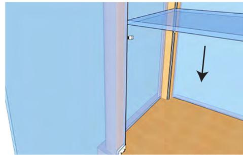
5. Push the plastic inserts into the top and bottom panel. Place the glass door holder (J) in place as shown below. Assemble all the holders on both sides, top and bottom.
