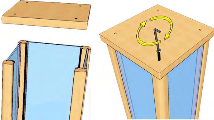
7. Assemble the door lock (H) by securing it on top of the glass door. Test the lock after assembling.
