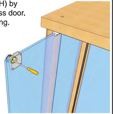
5. Push the plastic inserts into the top and bottom panel, and place the glass door holder (I) in place as shown below. Install the 2nd holder at the top the same way.
