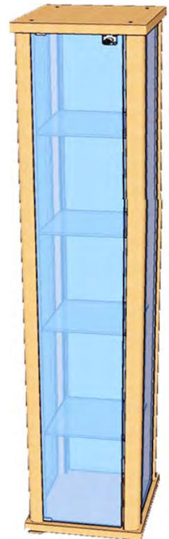
6. Carefully lift the glass door panel (D) and insert both ends into the metal brackets assembled in Step 5. Adjust the glass door to its best fit then tighten screws with screwdriver. *Tips: Open and close the glass panel to check if the door can move freely. Adjust as needed.*
