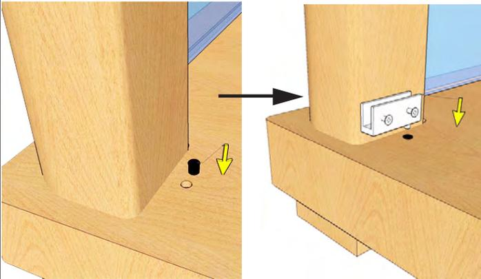
8. Adjust glass pegs on corner posts to desired height if needed. Be sure 4 pegs holding a glass shelf are on the same level. Carefully place 4 glass shelves on the pegs.
