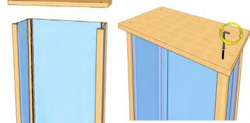
5. Push the plastic inserts into the top and bottom panel. Place the glass door holder (J) in place as shown below. Assemble all the holders on both sides, top and bottom.
