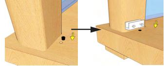
6. Carefully lift the glass door panel (D) and insert both ends of the back and side glass panels. into the metal brackets assembled in Step 5. Adjust the glass door to its best fit then tighten screws with screwdriver. The assembly is finished.
