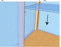
9. Insert the glass seal starting from 1 corner outside the display case. Apply silicon glass seal provided to all edges
