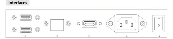
1. USB interface; 2. RJ45 interface(Ethernet); 3.HDMI input; 4.Power port; 5. On/Off button; Note: Please pull out the power plug before installing or disassembling the unit!
