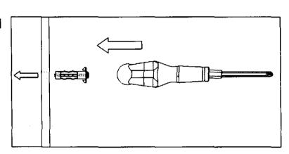
4-A) Press down firmly on the head of the screw with a screwdriver and turn the screw clockwise until the barrel crimps against the inside of the wall.
