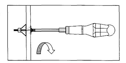
5) With the barrel pressing firmly against the inside of the wall, remove the screw by turning it counter-clockwise. If the wall anchor feels loose after removing the screw, re-insert the screw and tighten more.
