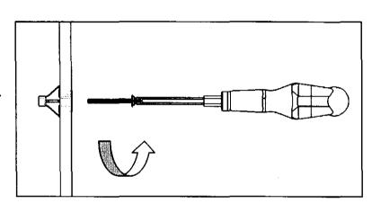
6) After the screws have been removed, line up the mounting holes on the rack with the wall anchors and re-insert the screws and tighten. (Be careful not to over tighten.)
