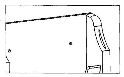
2) Using a power drill, drill a hole slightly larger than the barrel of the wall anchor.
