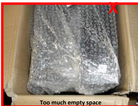
Too much empty space surrounding merchandise. Will allow it to shift while in transit.
