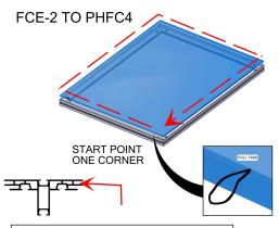
Install graphic by pressing the FCE-2 into the channels of PHFC4 extrusion. To pull graphics out of the channels, use tabs on the front side
