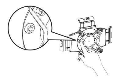
**B** How to unlock-To unlock the security lock by turning the key
