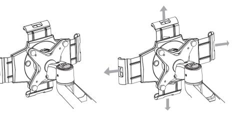
B To insert tablet in the right position and compress claw tight to fix tablet steady.
