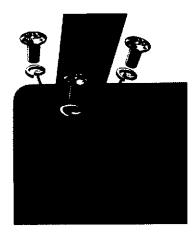
Insert 2 Phillips Screws(E) into the 2 inner Leg(B) holes as shown. Tighten with a Phillips Screwdriver.
