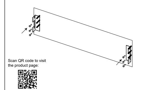
4. Carefully lift the bottle display shelf and hang it onto the brackets. Ask another person to help if necessary.
