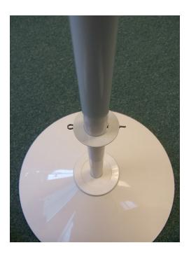
Step 4: Slide ball bearing onto the washer.
