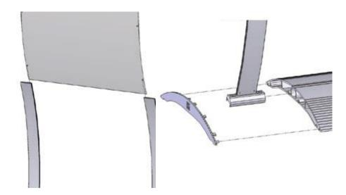
Remove end cap from base. Slide (2) side support into base and secure (1) in place with a screwdriver. Replace end cap. Keep the second extrusion loose to help install your poster. Use a measuring tape or the cross bar to estimate the width of your poster.
