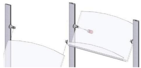
Insert each acrylic pocket into the brackets. Make sure your pocket is lying flush against the bracket to ensure a secure connection.
