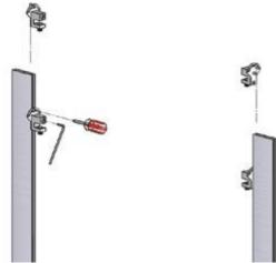
Measure the desired height for each shelf. Attach and secure each shelf bracket onto the side supports, using a Phillips Head screwdriver and the provided Allen wrench.
