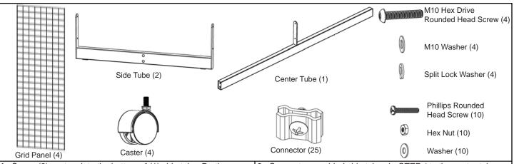
1. Screw (2) casters into the bottom of (1) side tube. Do the same for the other side tube.
