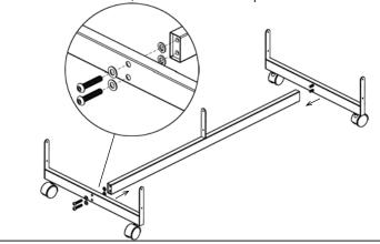
each side tube, fix them with phillips screws, hex nuts, and washers provided. Assemble another grid panel on the other side. Place another (2) grid panels onto the center tube,
