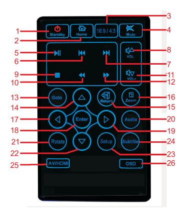
**1.Standby** Switches the Mini HD Player on and off from standby mode.
