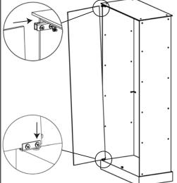
Assemble the other door the same way. Tips: Test the doors and adjust as needed.
