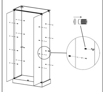
7. Carefully place 1 glass shelf (E) on the fixed pegs at the same level. Install the rest glass shelves the same way.
