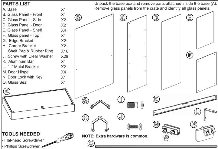
1. Place the base (A) on the ground, insert the front glass panel (B) and 1 side glass panel (C) into grooves in the base. Hold glass panels in place and connect them with edge bracket (G) and corner bracket (H) by using screws (J). Tighten screws with a flat-head screw driver. Do the same for the opposite side.
