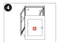
Fix the countertop by tightening the thumb screws on both sides as shown below.
