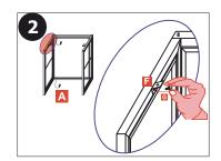
Carefully put the shelves inside through the door with its brackets hanging on side rails. Note: the finished edge of the shelf should face to the front.
