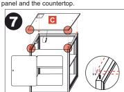
Place the door to the back of the main frame and align the holes on the brackets with insert nuts in the frame.
