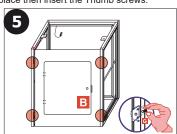
Assemble the SEG fabrics onto the main frame by inserting silicone edge into the slot on the front and sides.
